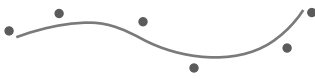
FIGURE 2 A set of six control points approximated with piecewise continuous polynomial sections.
