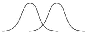
FIGURE 5 Two illuminated phosphor spots are distinguishable when their separation is greater than the diameter at which a spot intensity has fallen to 60 percent of maximum.
