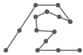
FIGURE 9 Applying this generator to the edges of an equilateral triangle produces a snowflake-filling Peano curve (also called a Peano space).
