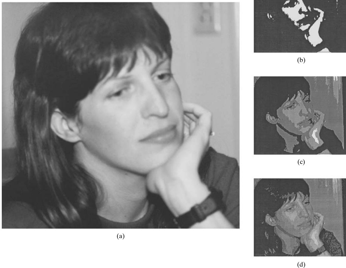
FIGURE 25 A continuous-tone photograph (a) printed with two intensity levels (b), four intensity levels (c), and eight intensity levels (d).
