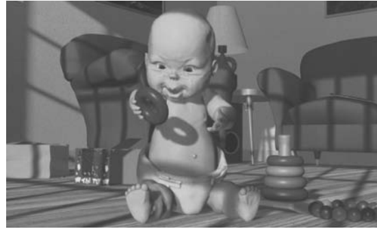
FIGURE 3 One frame from the short film Tin Toy , the first computer-animated film to win an Oscar. Designed using a key-frame animation system, the film also required extensive facial-expression modeling. Final images were rendered using procedural shading, self-shadowing techniques, motion blur, and texture mapping. (Courtesy of Pixar. © 1988 Pixar.)
